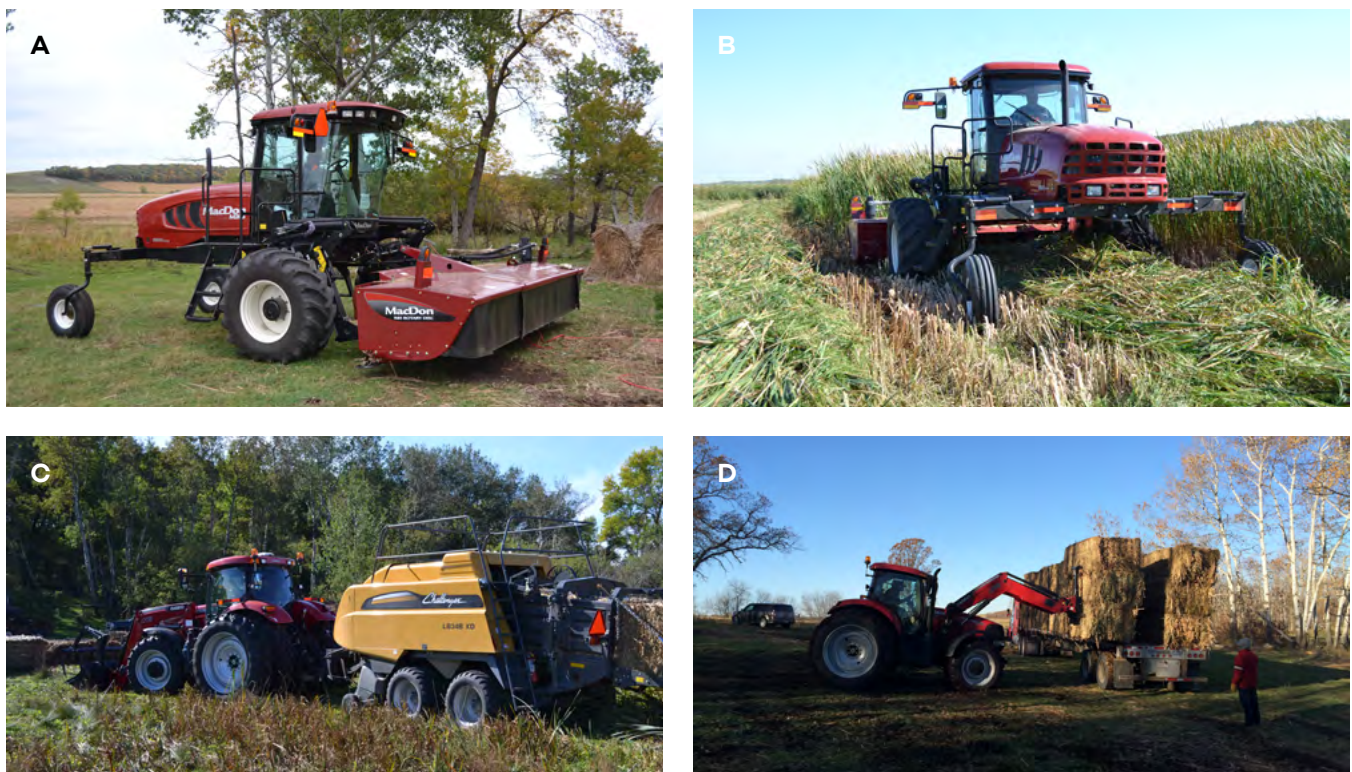
Figure 1. a) MacDon rotary disc mower conditioner, b) harvesting in Pelly's Lake, c) Case IH Puma 200 CVT tractor with a Challenger LB34B large rectangular baler, and d) shipping bales at Pelly's Lake.
