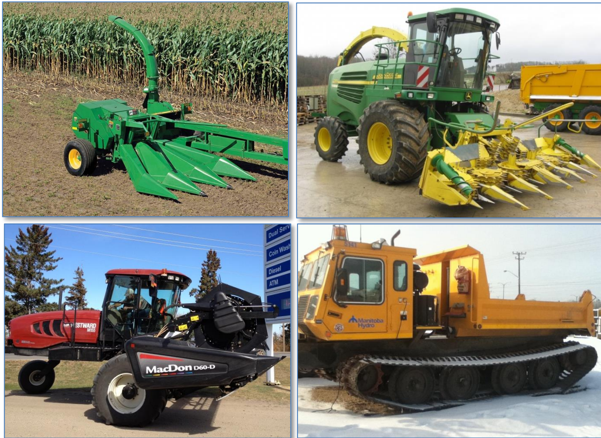
FIGURE 19. Clockwise from upper left: pull-behind forager harvester with PTO attachment; self-propelled forage harvester with rotary corn silage header; tracked collection vehicle with dump box; and self-propelled swather.
