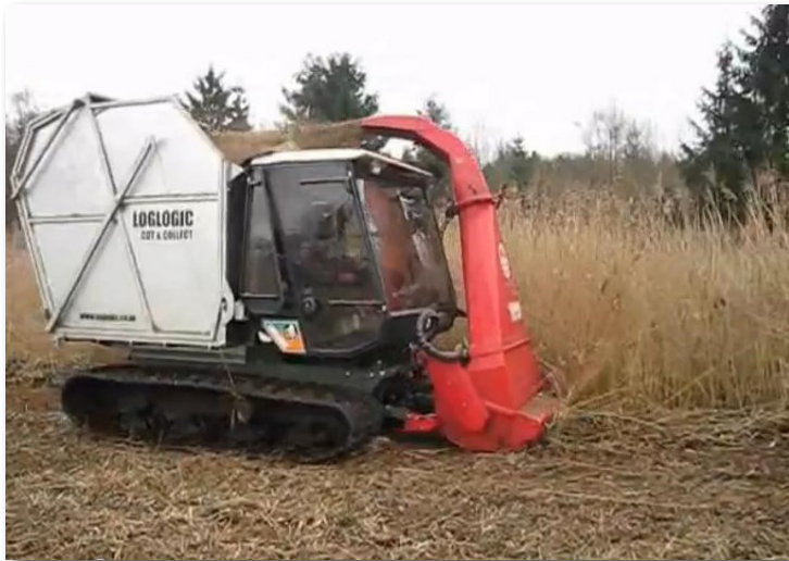
Softrak low ground pressure tracked vehicle – “Cut and collect system”
