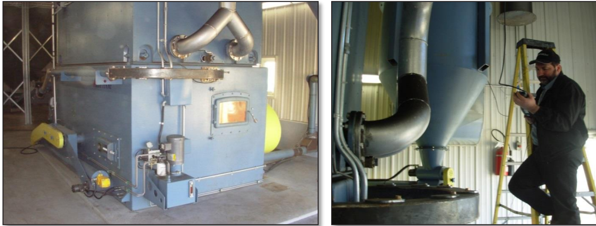
FIGURE 22. The Blue Flame Stoker biomass burner in use at the Sturgeon Creek Hutterite colony for cattail biomass burn trials (Grosshans et al., 2011a).
